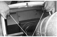
*Latches* 3) Lift the Glass Front Assembly up.
